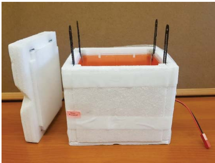
Prototype of new chilled adult mosquito release device for ground and aerial release of sterile males.
