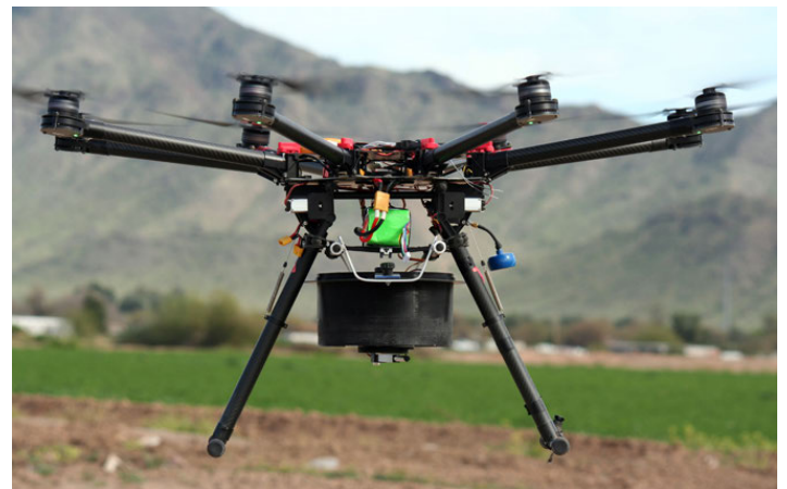
A specially designed drone for dropping sterilized moths on infested orchards is being tested in the Okanagan. The device can hold enough moths for around 40 acres, which it can cover in 8 minutes. Image Credit: M3 Consulting Group.
