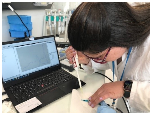
FIG. 4. Ms Rezende applying 50 \mu L of spiked turmeric tea to the SPE electrodes, connected via a transducer to the potentiostat.
