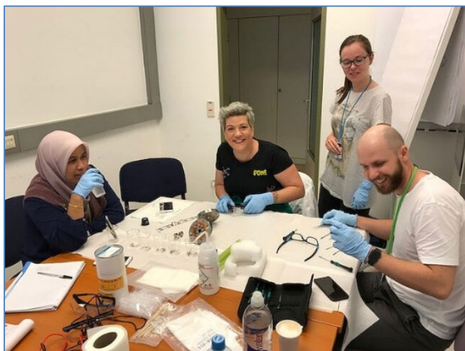
'FoodIntegrity' trainees dismantling and cleaning a Nier-type electron impact ion source.
