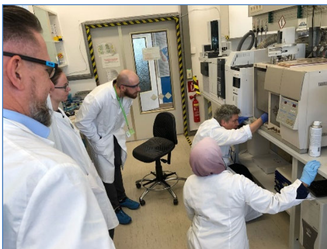
'FoodIntegrity' trainees fitting combustion and reduction tubes to in an elemental analyser.
