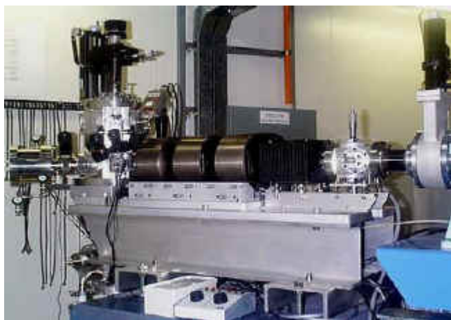
Nuclear Microprobe end station showing the vacuum chamber, quadrupole triplet, scanning magnet and the collimating slits.
