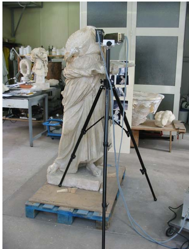
Fig. 1. EDXRF measurements for the indoor ancient roman statue "La fanciulla di Anzio"
