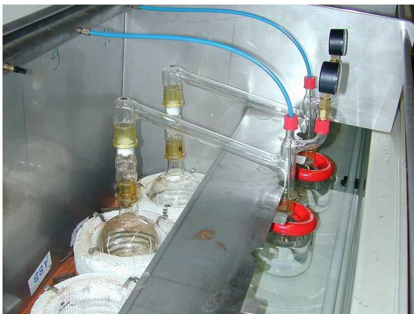
Left side: heater with glass bulb for original sample; above visible the white glass wool; right side: glass bottle in water cooling bath with red lead ring (against buoyancy); above visible the blue vacuum hose with steel capillary (0.2mm in diameter) and at the right side a manometer as leak detector.
