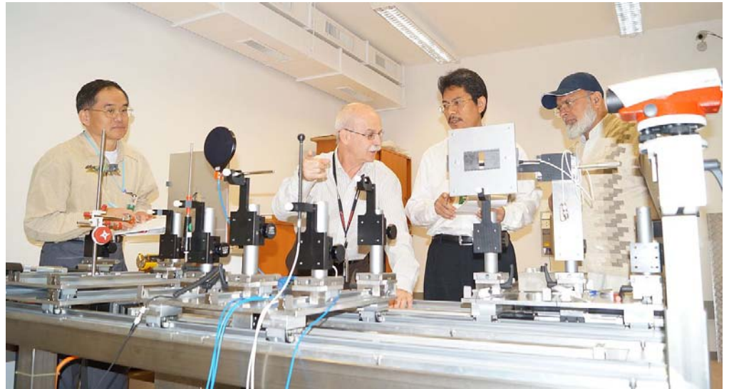
Participants positioning ionization chambers during the Technical Meeting on Dosimetry and Comparisons in Diagnostic Radiology held at the IAEA Dosimetry Laboratory.
