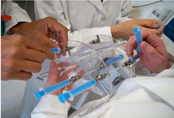
Figure 2: Preparation of the triple line insert for tomographic spatial resolution measurements.
