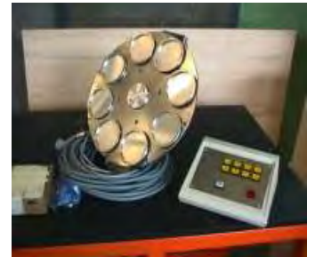
A half-value layer measurement system for X ray beams and its automatic filter wheel.
