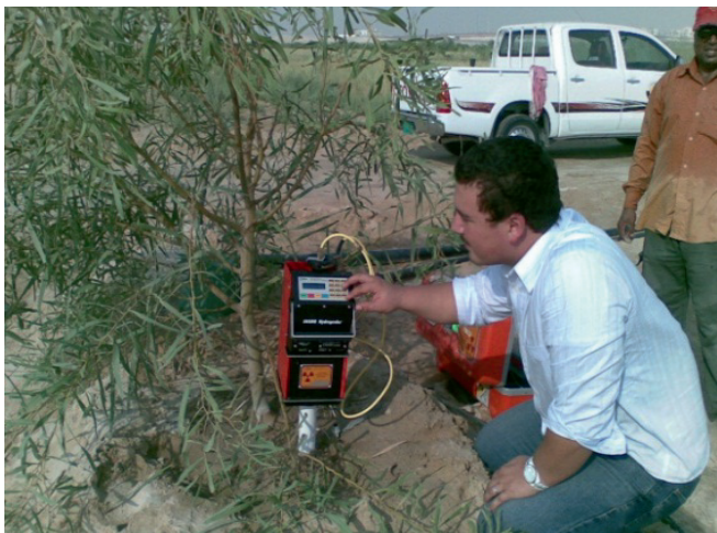
Fig. 4. The soil moisture neutron probe is used to measure soil moisture status and to assist with drip irrigation scheduling for vegetable crops and salt-tolerant Acacia bush plants ( Acacia Amphlicepts ) in Kenya (top) and Qatar (bottom), respectively.
