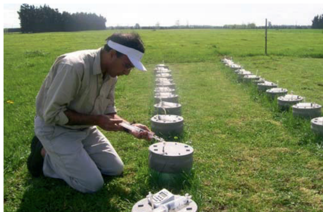
Fig. 6. Gas released from farmlands collected for determining greenhouse gas (GHG) emissions.
