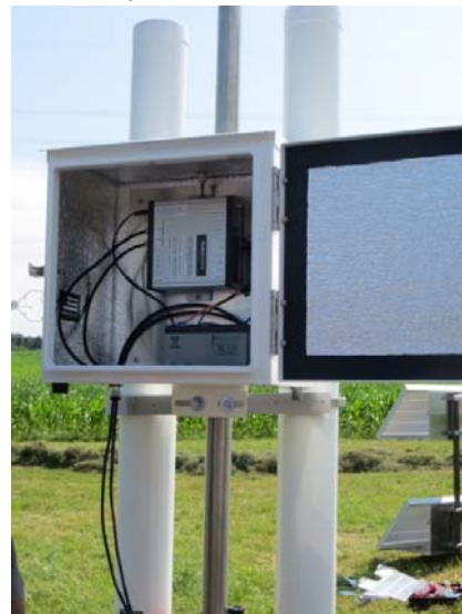
The CRS 1000/B model cosmic ray neutron probe
