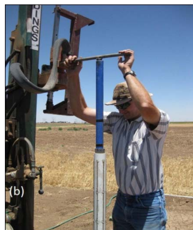
Fig.1. Installation of a stack of 20 cm long WOAT sensors into undisturbed soil by augering from within between alternative pushes with a hydraulic coring machine (Giddings).
