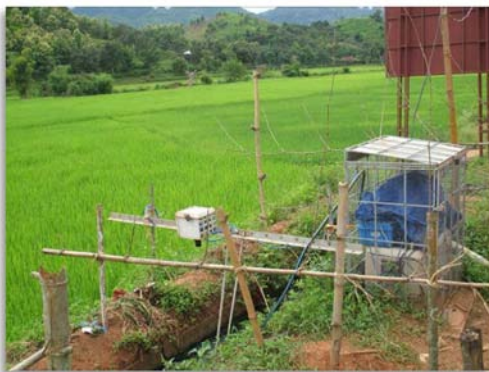
A water flow measuring device and automatic water sampler in a lowland irrigation channel (Courtesy: University of Hohenheim)
