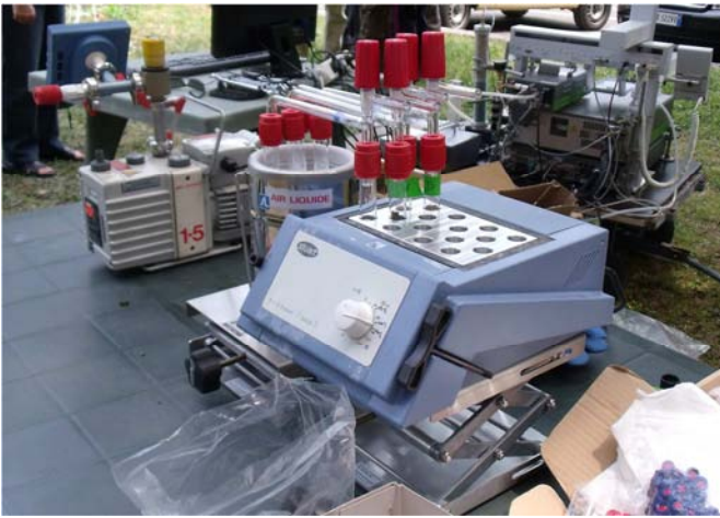
Fig. 1. Portable vacuum extraction distillation equipment in field operation
