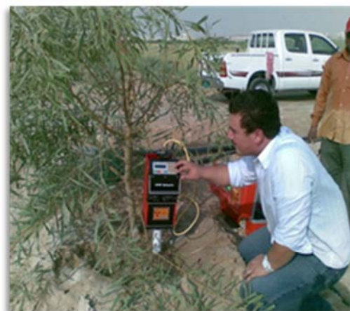
Soil moisture is measured using the soil moisture neutron probe.
