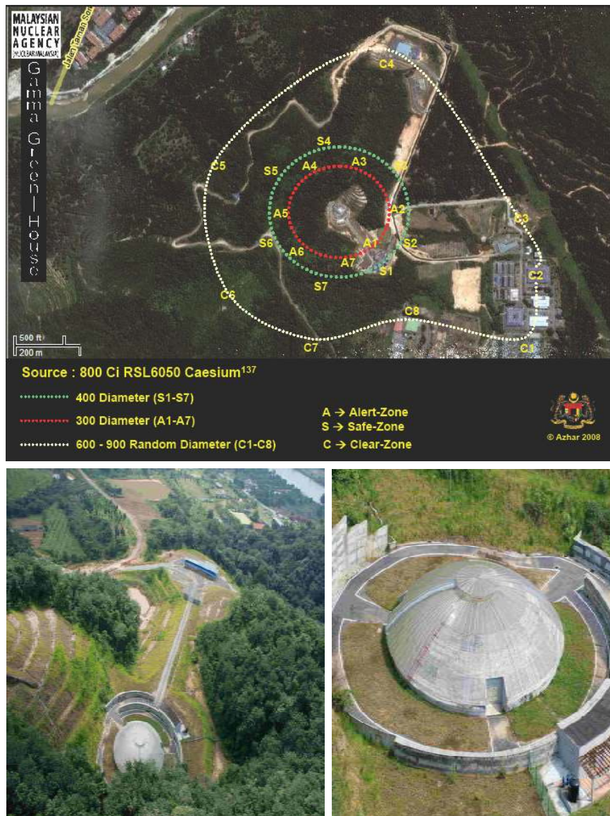
Figure 1. Malaysian nuclear agency gamma greenhouse a) Schematic view of the facility with different safety levels, b) birds view of the facility and surrounding area, c) a full view of the gamma greenhouse.
