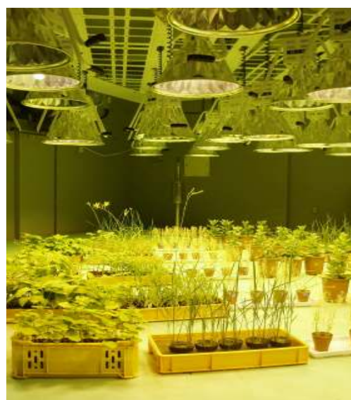
Figure 2. The inner part of irradiation room in gamma phytotron. Light source can be controlled up and down for the optimum light intensity.
