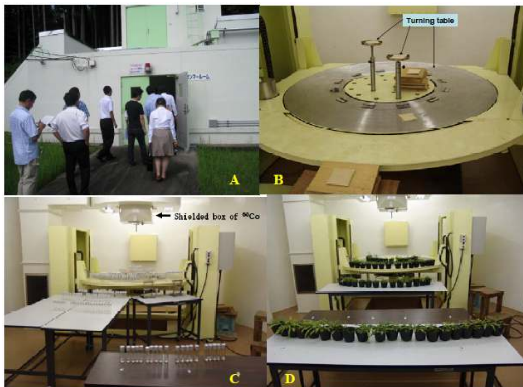
Figure 2. A) A building of gamma room for acute irradiation. B) Irradiation to seeds C) to in vitro materials D) and to plants. (Photos courtesy of Toshikazu Morishita, IRB, NIAS)
