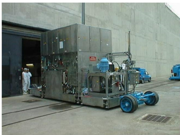
Figure 2. Mobile System for polymer encapsulation of ion exchange resins (Courtesy: SOCODEI, France)
