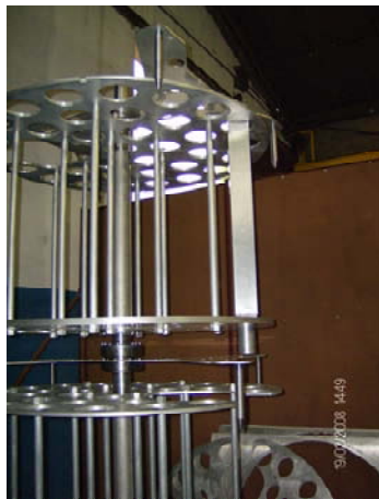
Figure 2 – Stacked spools with a dummy fuel assembly
