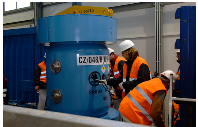
Prague Czech Republic – preparing a cask loaded with spent highly enriched research reactor fuel for transport to the Russian Federation
