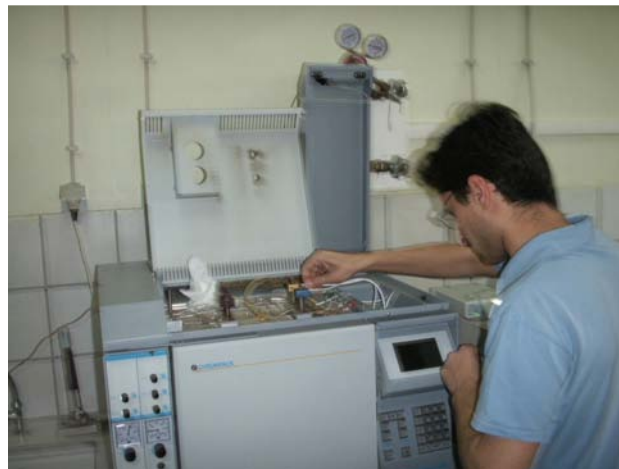
Picture 1: Mr. Enis Darilmaz (from Izmir laboratory) helping with the connection of the electrode to the electron capture detector.
