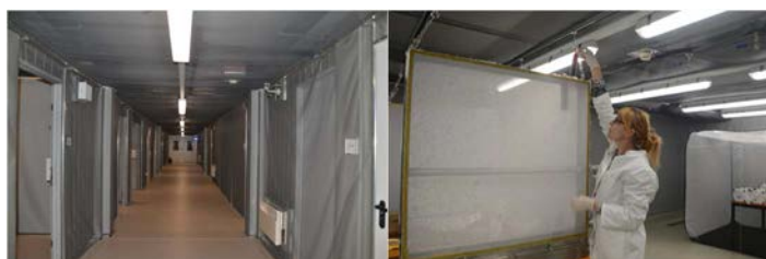
Left: main corridor of the container refurbished into an insectarium, giving access to 13 rooms corresponding to a 264 m 2 confined working space. Right: blood feeding of Aedes spp. mosquitoes in the reference FAO/IAEA mass-rearing cage.
