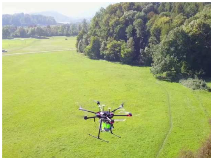
Field test of a drone equipped with a mosquito release machine.
