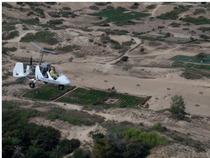
The gyrocopter equipped with the newly developed chilled adult release system that is now routinely being used to release sterile male Glossina palpalis gambiensis over the Niayes.
