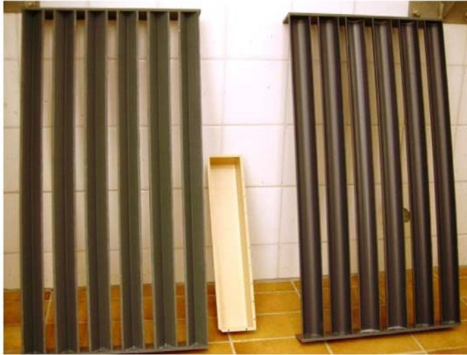
New olive fly larval diet trays under evaluation (left with straight grooves and right with curved grooves). In the middle, the standard diet tray.
