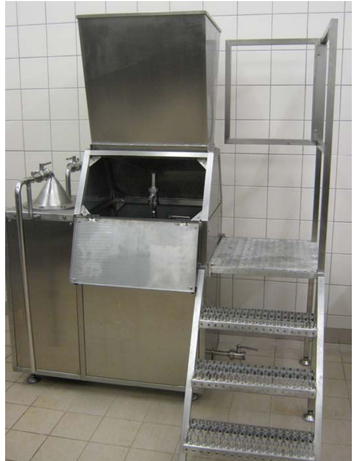
Larvae-pupae separator made of stainless steel.
