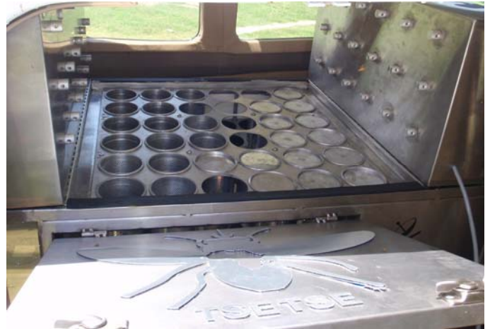
Chill release machine mounted in a Cessna 206 with the top open to show 30 of 36 cylinders mounted. The cylinders on the left side have released their flies to the main funnel below.
