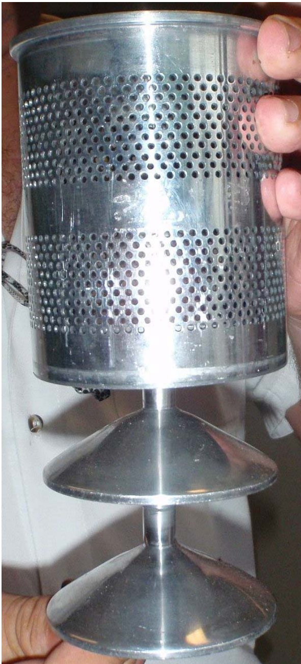
Fly holding cylinder showing the mechanism to release the flies into the main funnel lowered. The cylinder is perforated to permit chilled air circulation.
