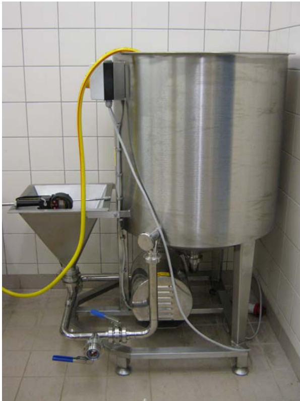
Larval diet mixer machine with the dispenser feeder.
