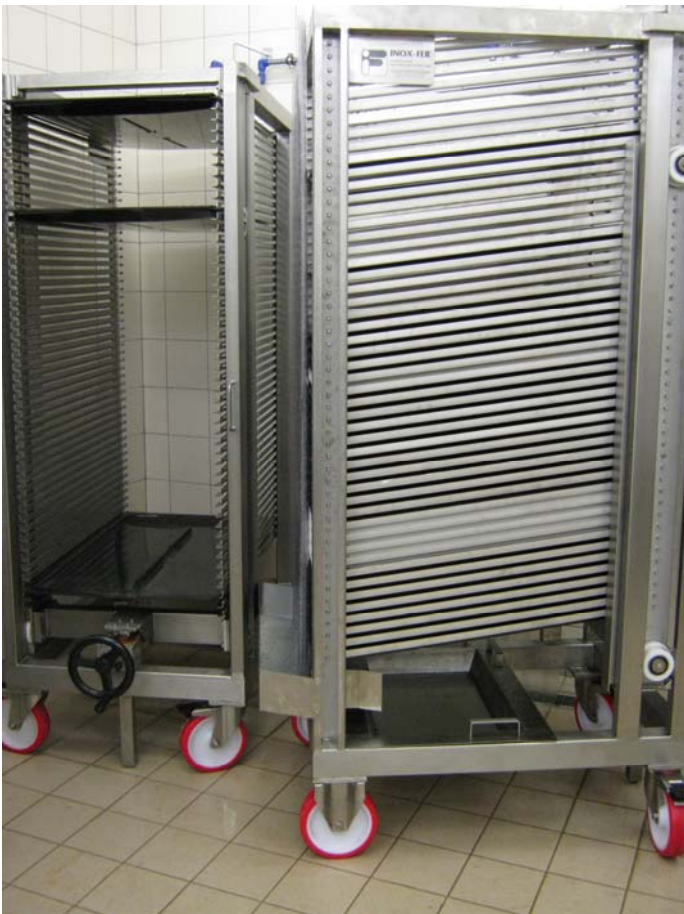
Mosquito rack system. The plastic panel, the slide and the collector of the immature stages from the larval trays on the right.
