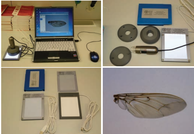
(upper, left) The Dino-Lite AM413 handheld digital microscope connected to a laptop, (upper, right) components of the unit, (lower, left) the LED light source, and (lower, right) a picture of a wing of G. brevipalpis, taken with the microscope.
