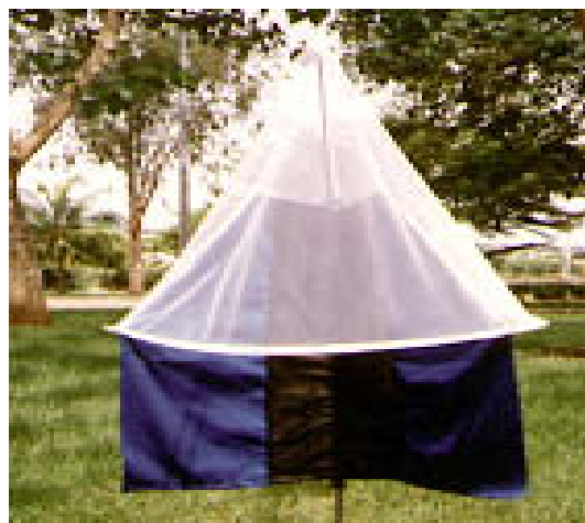
Fig. 7: Insecticide-impregnated Vavoua trap, used for the reduction of the Gpg population in the Niger River Basin in Mali
