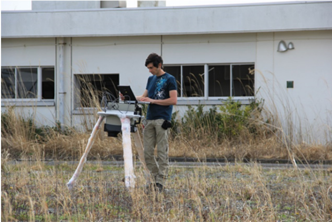
A member of the Institut de Radioprotection et Sûreté Nucléaire (IRSN) prepares to carry out in-situ gamma spectrometry measurement exercises during the Fukushima workshop (Photo Credit: P. Kenny/IAEA-IEC)
