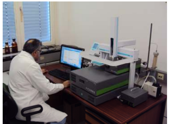
Figure 1. The cavity-ring-down spectroscopy isotopic analyser installed in the FEPL.
