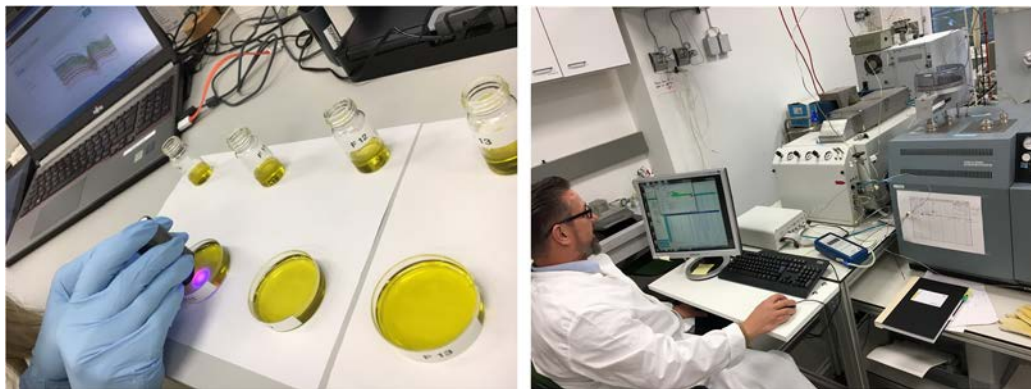
Screening of foods for authenticity using cheap, hand-held infra-red sensors (left) with further investigation of suspect samples by confirmatory nuclear techniques such as isotope ratio mass spectrometry (right) makes the technology accessible for a variety of user and Member States.
