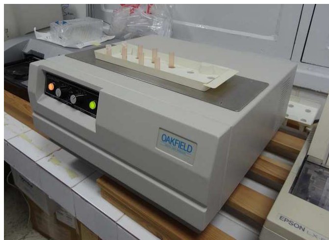
Gamma counter for measuring ^{125}I .
