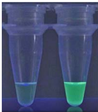
Visible colour changes in reaction tubes allow discrimination of positive and negative results when using the LAMP-PCR for diagnosing avian influenza
