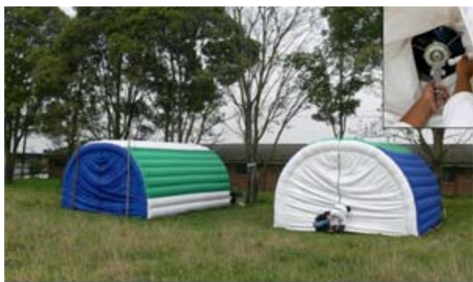
Polytunnel chambers fitted around animal cages used to measure methane production in Colombia. Inset: Sampling of gases within the chambers (Photo courtesy: Ms. Olga Mayorga)
