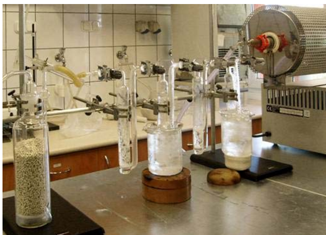
Carbolite: automatic combustion system for ^3\text{H} and ^{14}\text{C} sample preparation
