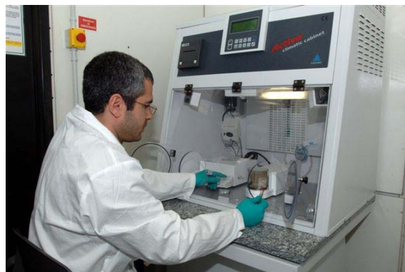
Filter weighing to determine the net mass gain on airborne particulate matter <math><10\ \mu\text{m}</math>
