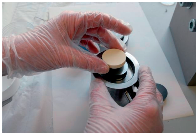
Preparation of a spiked milk powder reference material
