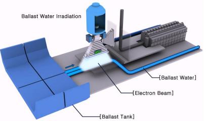
Radiation technology has applied for ballast water treatments by free radical formation to prevent the transfer of invasive organisms.
