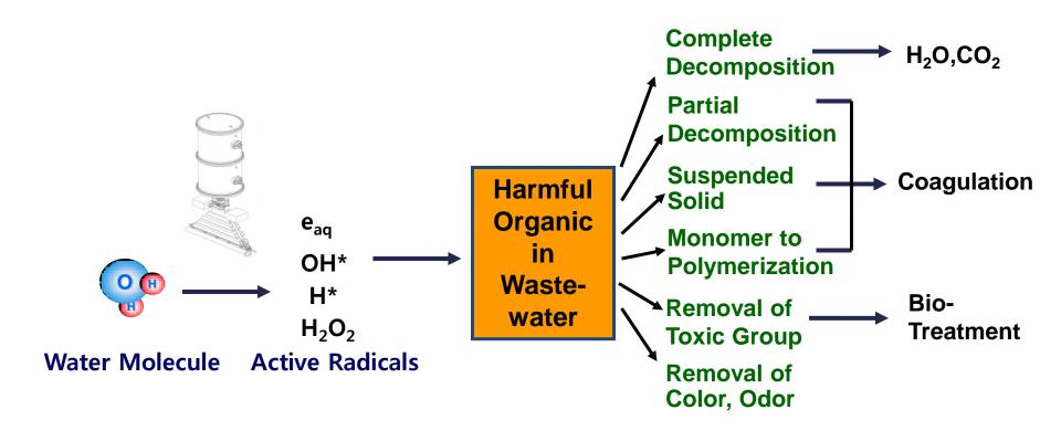
Ionization and excitation of water molecule by radiation produces free radical to treat liquid wastes
