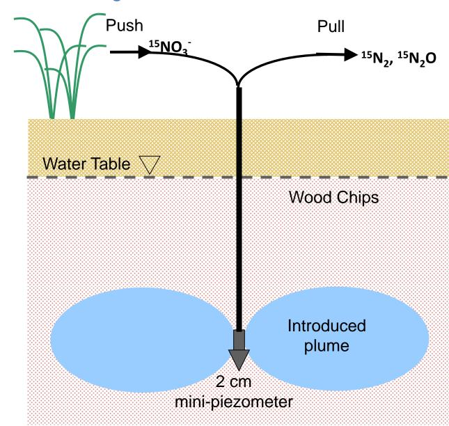
Push-Pull <sup>15</sup>N method shows denitrification is the main mechanism for nitrate removal (Acetylene-block
