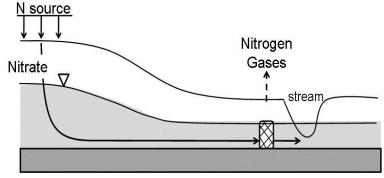
In deep aquifers, substantial nitrate can bypass wall bioreactor
