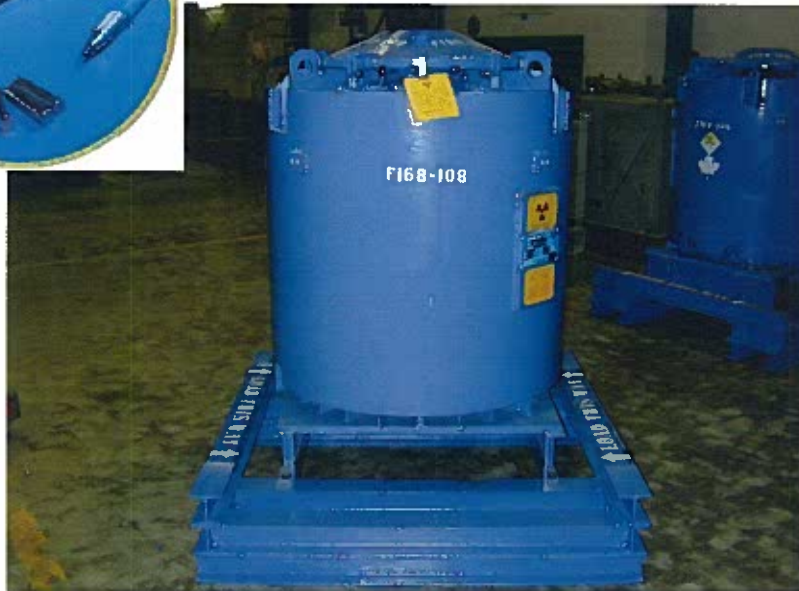
Sealed source pencils: approx. 0.5" diameter x 18" length
