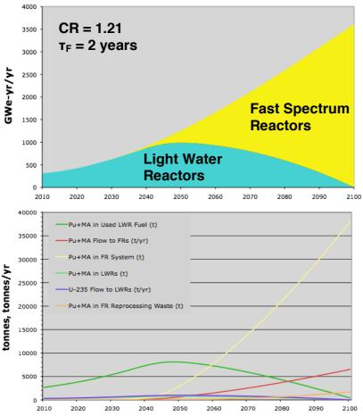
FIG. 2a, b. Power production and stocks and flows of Pu + MA and  $^{235}U$  for fast-spectrum reactors.
