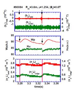
Fig.6 Time evolutions of magnetic fluctuations of TAE and RIC,  $W_p$ ,  $H_{\omega}$  and line-integrated electron densities at the magnetic axis and the edge, in a high beta plasma where a transient confinement improvement is triggered by TAE bursts.
