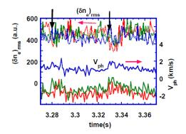
Fig.8 Time evolutions of density fluctuation amplitude and the phase velocity measured with  $CO_2$  laser phase contrast imaging. Every TAE burst shown by vertical arrows, the phase velocity is enhanced in the ion diamagnetic drift direction.
