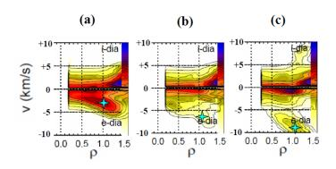
Fig.3 Amplitude and phase velocity v of electron density fluctuations measured by  $CO_2$  laser phase contrast imaging technique as a function of the normalized minor radius, at the L phase (a) and H-phases (b) and (c). The time windows at the three cases are respectively set as (a) $\Delta t_{LH}$ =-30ms  $\sim$  -20ms, (b) +20ms $\sim$ +30ms and (c) +130ms  $\sim$  +140ms. The characteristic fluctuation peak propagates in the electron diamagnetic drift direction is marked with a blue cross.
