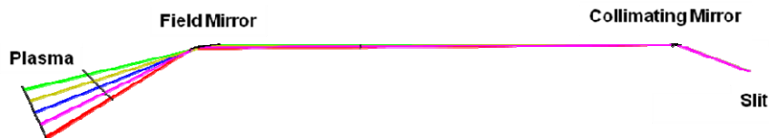
FIG. 2. Backward ray-tracing from the slit of the spectrometer to the plasma edge region.
