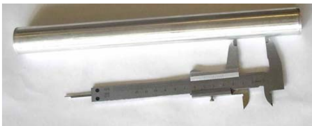
FIG.5. Photograph of the neutron attenuator
