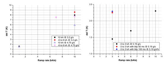
FIG. 7. Relationship between current ramp rate and temperature rise in PF1L (left) and PF2L (right)
