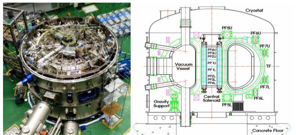
FIG.2. KSTAR magnet system
