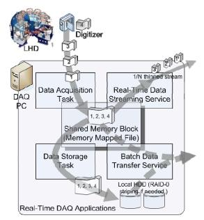
FIG. 2. Inside diagram of streaming DAQ: All the data blocks are handled on the volatile random access memory (RAM) [5]. The sub-shot data files will be newly made and closed every 10 seconds so that any data clients can refer them even if the RT DAQ is still continuing.
