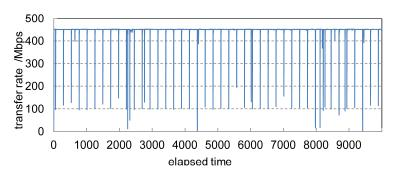
FIG. 6. Result of Japan-US bandwidth test between NIFS and GA, San Diego, CA: With the limited forwarding rate of 460 Mbps, very stable 451 Mbps throughput was obtained over 10 000 s. The comb-like drops are considered due to some periodical task awoken on the receiver computer.
