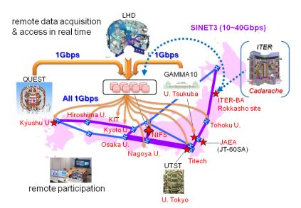
FIG. 4. Multi-site data platform on SNET: All the diagnostic data of each device are migrated into main storage in RT, and then delivered to every remote and local site.
