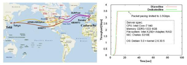
FIG. 5. Results of Japan-France bandwidth test: The fiber distance is about 15 000 km whose round-trip latency time is about 310 ms. Between 10 Gbps ports at both ends, the bandwidth was limited to 4 Gbps for the 10 Gbps shared backbone; SINET3, GEANT2, and Renater. The dedicated path through APAN/JGN2plus and SURFnet was also used.
