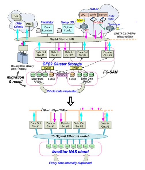
FIG. 3. Schematic view of the LABCOM DAQ and store system: The storage cluster had a mirrored structure on FibreChannel storage area network (FC-SAN) to store replicated files previously (left). They are replaced by distributed network attached storages (NAS) named "IznaStor" in 2010.
