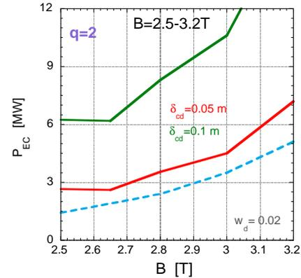
**FIG. 2:** EC power needed for suppression of the (2,1) mode. Dashed line corresponds to the driven current widths  $\delta_{cd}$  computed by beam-tracing; solid lines to the fixed values  $\delta_{cd} = 0.05$  and  $0.1$  m.
