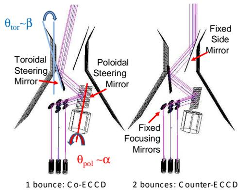
**FIG. 6:** sketch of one module (6 wave beams) the JET EC launcher (top view)
