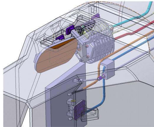
**FIG. 7:** preliminary design of the JET launcher: mirrors for poloidal and toroidal steering.
