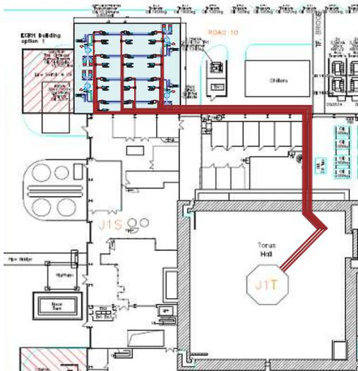
**FIG. 4:** sketch of the plant layout and waveguide routing from the gyrotron building to the tokamak
