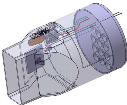
**FIG. 8:** preliminary design of the JET launcher: outer structure of the plug-in unit
