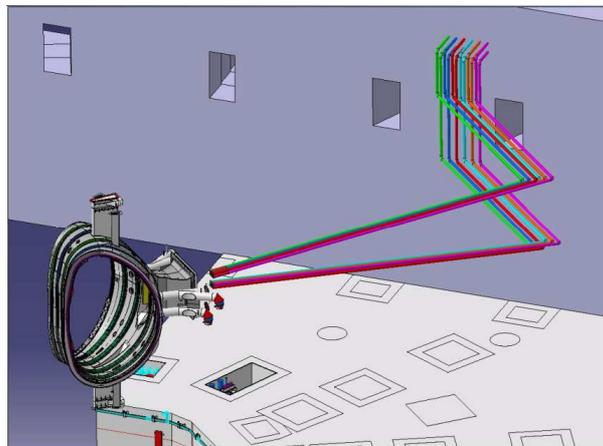
**FIG. 5:** preliminary design of the waveguide system in the JET Torus Hall, from the North wall to Octant 2.
