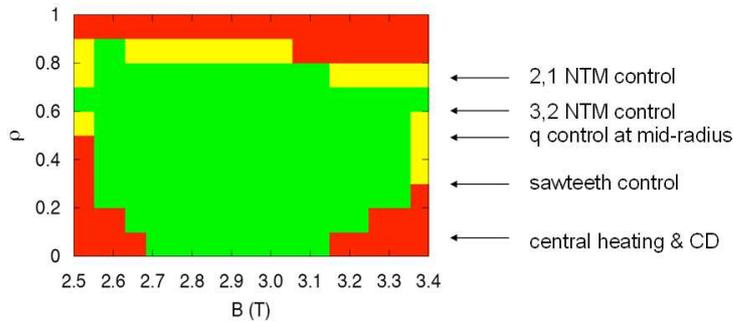
**FIG. 1:** Operation diagram for a JET ECRH system at 170 GHz, computed for a reference H-mode scenario. Green means that the envisaged functions (listed on the right) are possible, red not possible, yellow marginally possible
