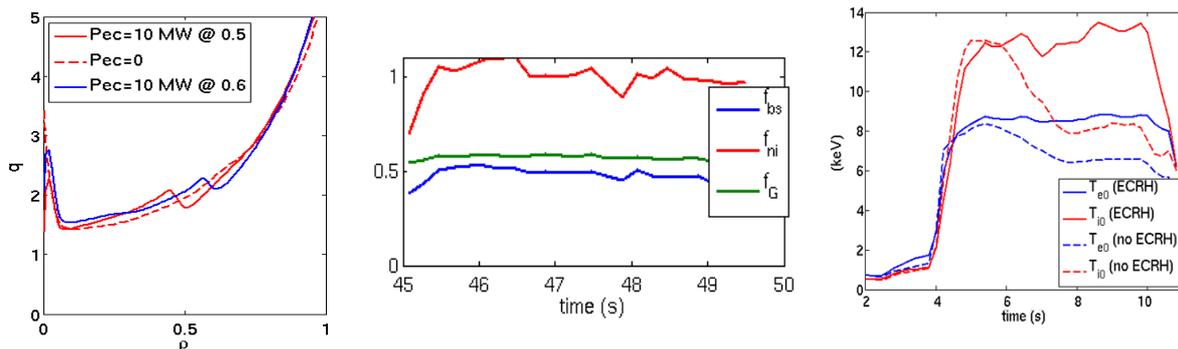
**FIG. 3:** Predictive simulations of a JET advanced scenario by the CRONOS code. Left: safety factor without and with ECCD at two different locations ( $\rho \sim 0.5$  and  $0.6$ ). Middle: bootstrap, non-inductive and Greenwald fractions vs time, with ECCD at  $\rho \sim 0.6$ . Right: time evolution of electron and ion temperatures with and without ECCD at  $\rho \sim 0.6$ . ( $B_0 = 2.7$  T,  $I_p = 1.8$  MA,  $P_{NBI} = 22.5$  MW,  $P_{ICRH} = 6.5$  MW,  $P_{LH} = 2$  MW)
