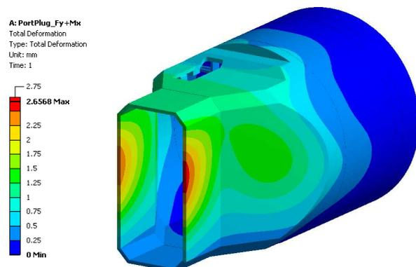
**FIG. 9:** Total deformation of the plug (in mm) due to e.m. forces: IMN force in toroidal direction and a IMNm moment in radial direction (Finite Element simulation)
