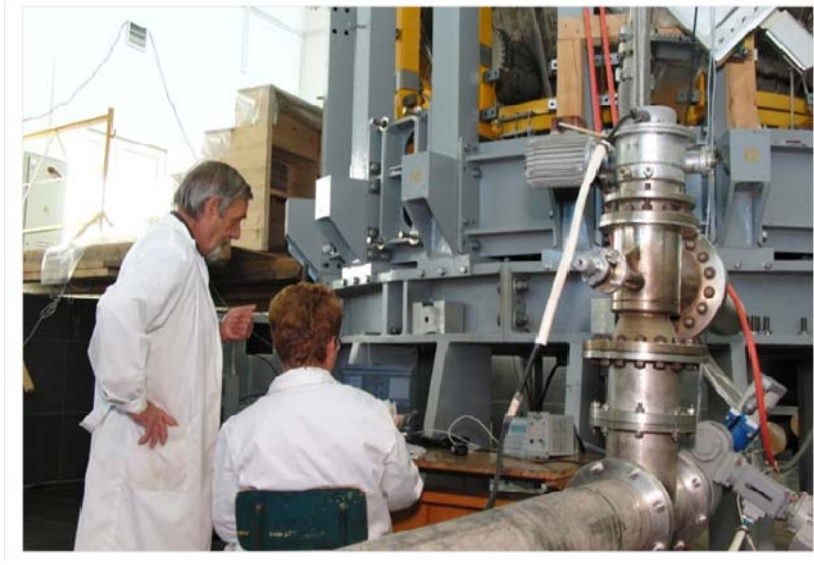
FIG. 1. Pumping of KTM vacuum chamber
