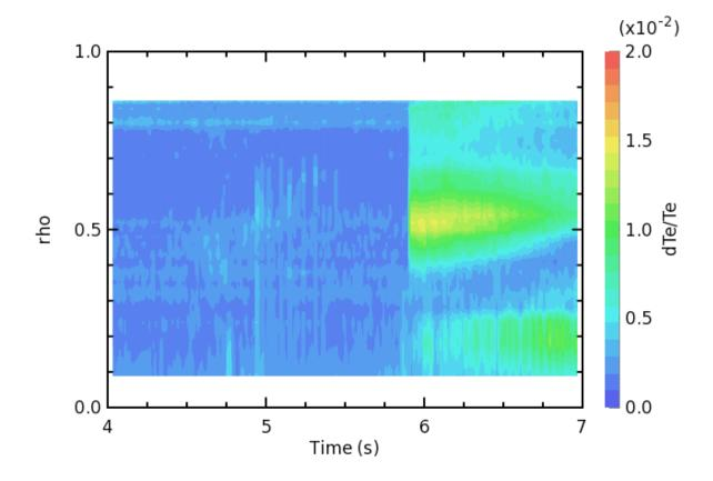
*Fig.3 Contour of amplitude of fluctuation of electron temperature in the frequency range of* 0.4 - 1.4kHz *measured with ECE.*
