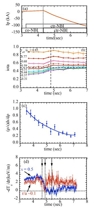
Fig.1 Time evolution of (a)toroidal net current, (b) rotational transform, (c) magnetic shear and (d) electron temperature gradient at a rational surface of  $\iota = 0.5$  and near the magnetic axis  $r_{eff}/a_{99} \sim 0.1$ ) in the discharge, where the direction of NBI switched from balance to counter to equivalent plasma current at t = 4.3s.
