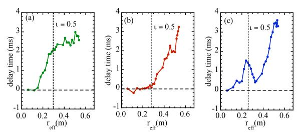
Fig.5 Radial profile of time delay of the heat pulse due to the modulated ECH in the plasma with (a) no magnetic island (t=4.7s), (b) stochastic region (t=4.9s) and (c) m/n=2/1 magnetic island (near the O-point) (at t= 5.4s). The locations of rational surface of  $\iota = 0.5$  are indicated with dashed lines.
