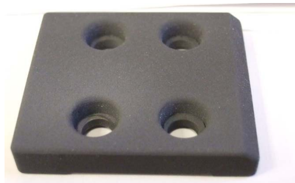
Figure 8: Unexposed RF protection molybdenum tile coated with \sim 100 \mu\text{m} of boron. The boron film is porous and was approximately 50% theoretical density.
