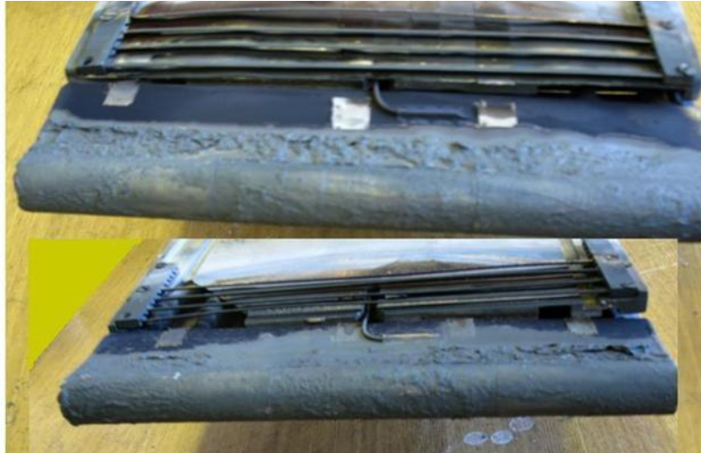
FIG.4. Head of “W-Li” limiter after exposition in 1000 shots of T-11M, e-side (top) and i-side (down).
