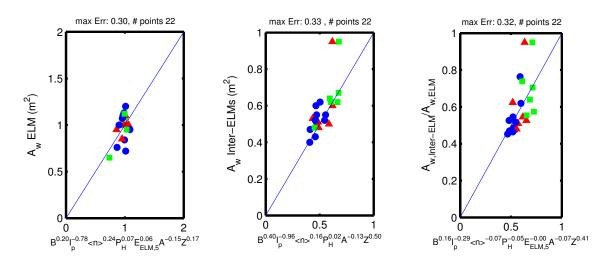
Figure 5: IR-measured wetted areas,  $A_W[m^2]$ , during ELM (left), inter-ELM (middle) and their ratio (right) vs best-fit scalings with field, current, density, heating power, A and Z (and for ELM quantities also with ELM deposited energy) for all ion species.
