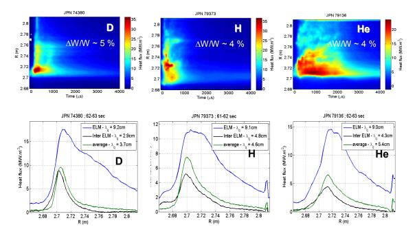
Figure 3: Radial heat load profiles on the outer divertor target in comparable D, H and He plasmas. The bottom frames show inter-ELM, ELM and average profiles and their corresponding integral widths. The top frames show the temporal evolution of the heat load profiles during a typical, medium sized ELMs ( $\Delta W_{ELM}/W_{dia} \sim 4$ -5%).
