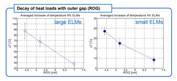
Figure 2: ELM heat load interation with outer limiter for two D discharges, with relative ELM size,  $(\Delta W_{ELM}/W_{dia})$  of 9% (left) and 4% (right), for different values of the outer gap (ROG)
