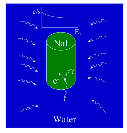
Taking into account the typical interactions in the water, in the material of the housing and in the NaI crystal.
