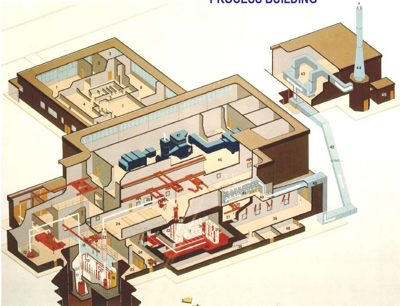
**GROUND FLOOR:** hot cell, “warm” cell, decontamination cell, fuel pool, control room, the labs, the offices, etc.
