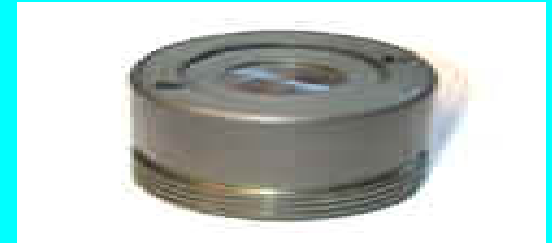
^{241}\text{Am}/\text{Be} research source
