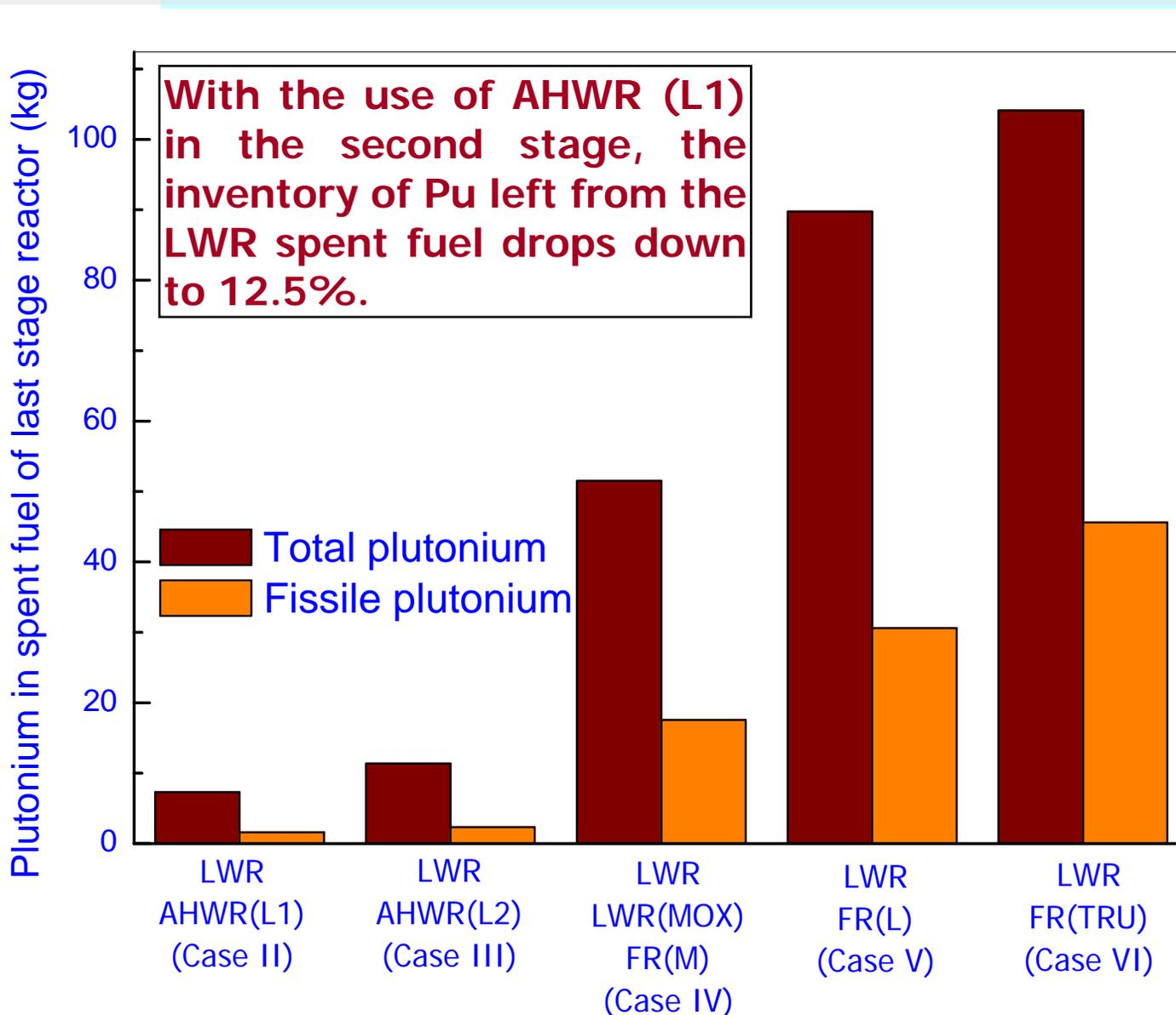
Total Pu from the LWR spent fuel used in an AHWR based configuration results in far less plutonium in spent fuel than when used in FR based configurations.
