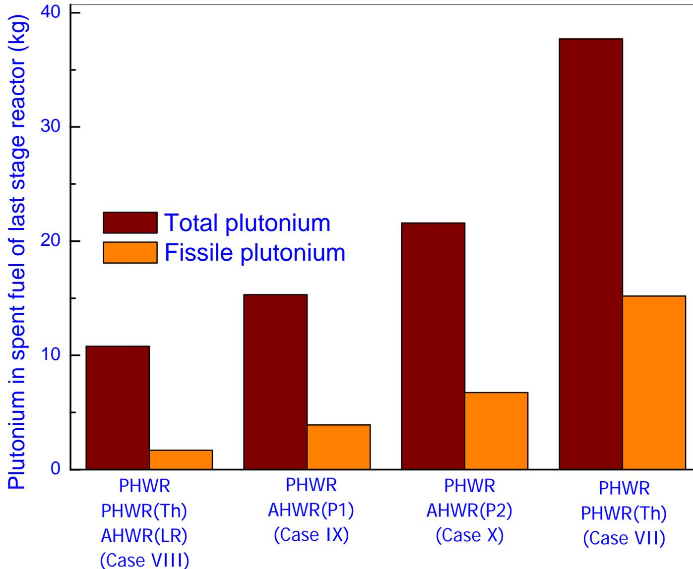
The multiple cases for thorium utilisation with different characteristics exhibit the flexibilities available with the use of thorium in conventional thermal reactors or in thermal reactors using conventional technologies
