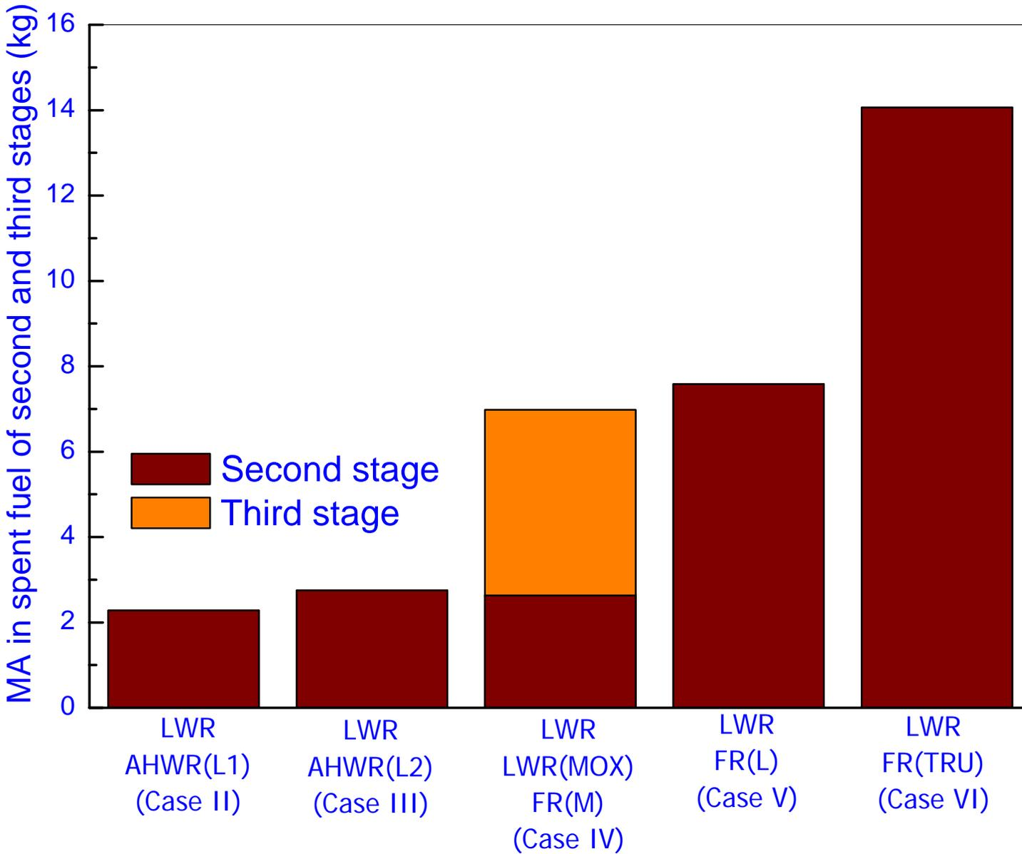
AHWR based options produce substantially reduced quantity of MA as compared to that produced with FRs.
