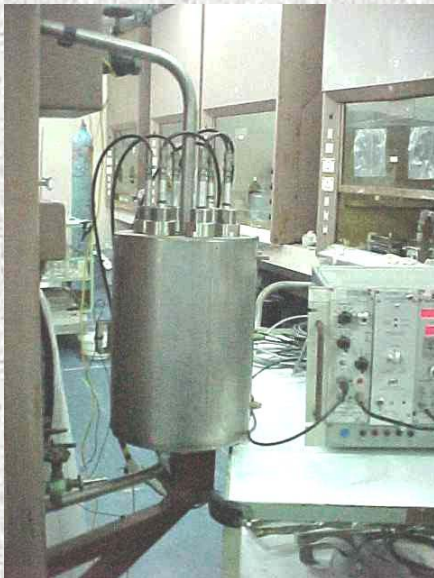
Neutron collar for on-line monitoring
