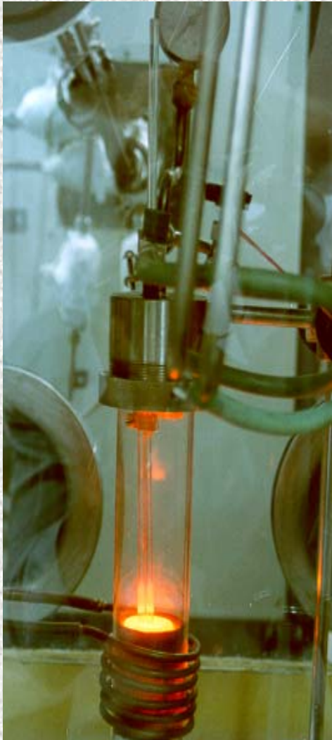
Injection casting in Glove Box
