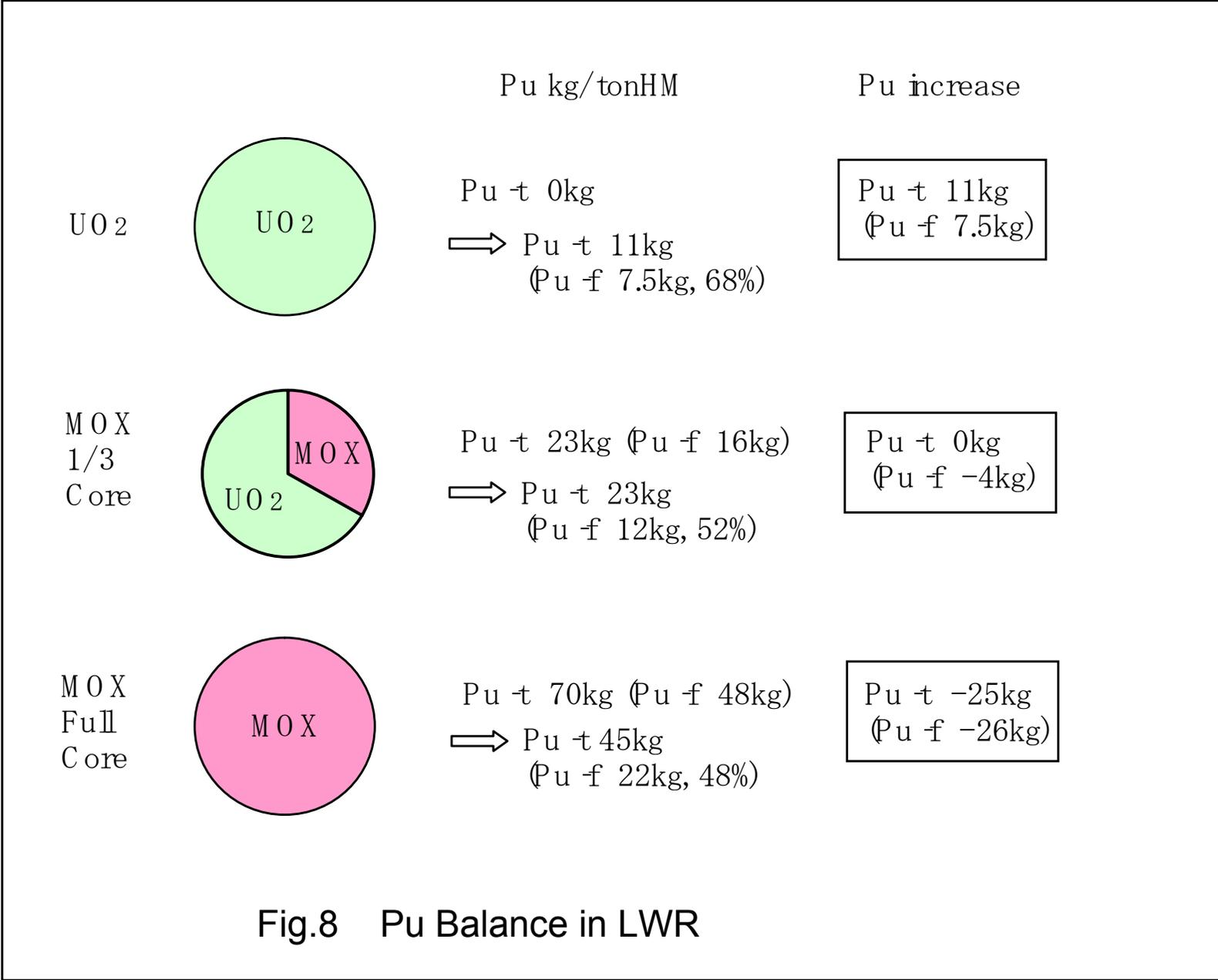
Fig.8 Pu Balance in LWR
