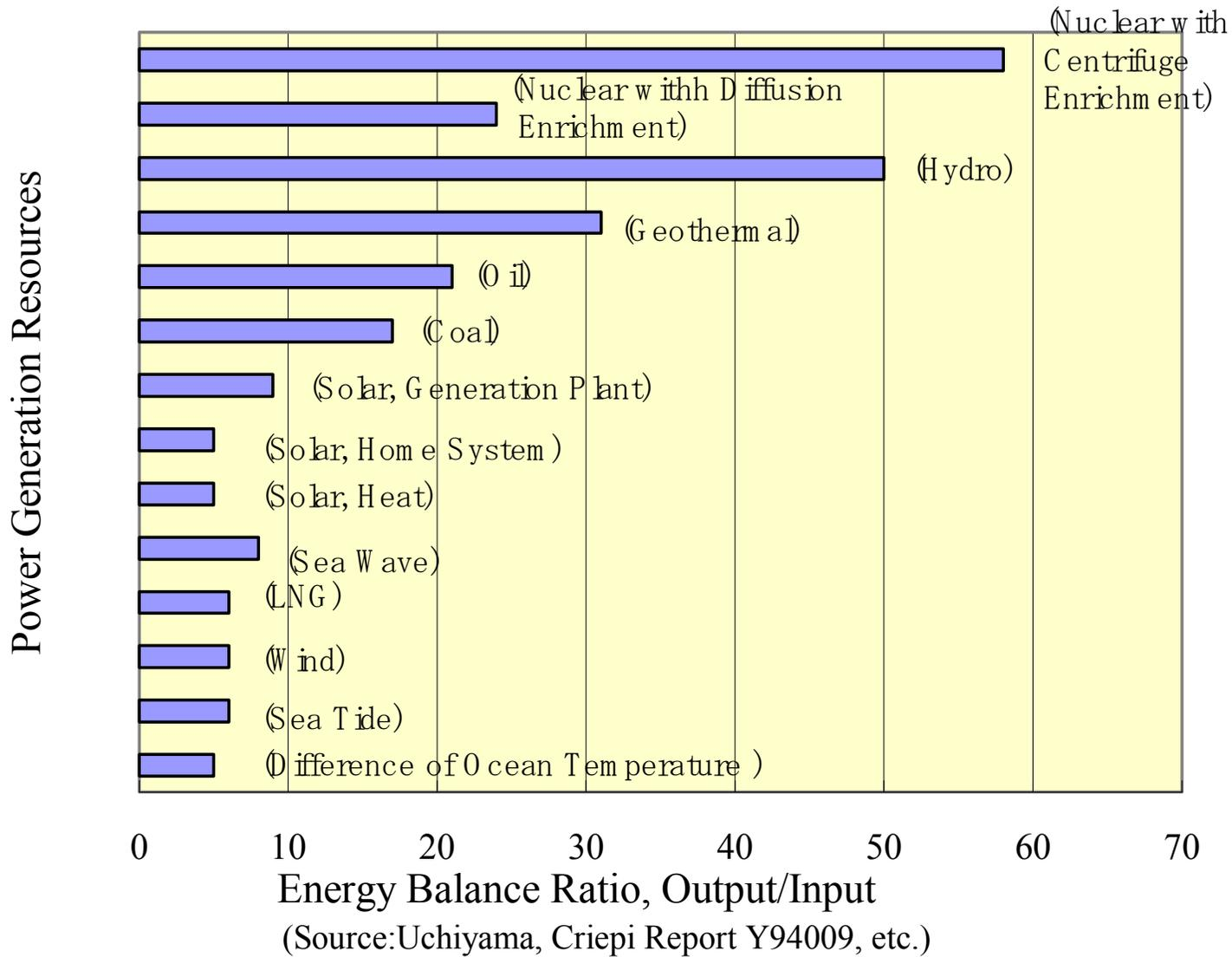
Fig.2 Energy Balance Ratio of Various Generation System in Japan
