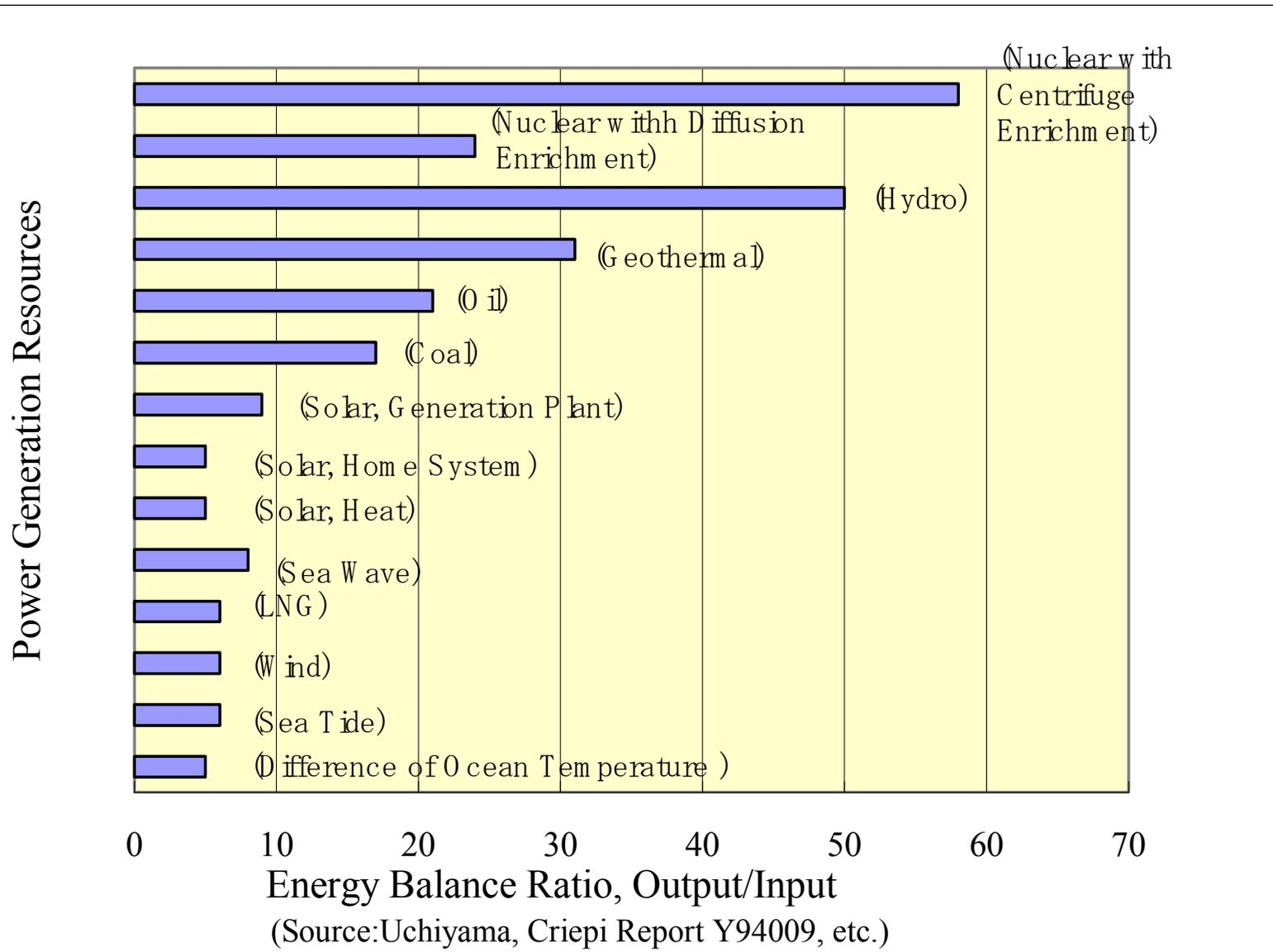
Fig.2 Energy Balance Ratio of Various Generation System in Japan
