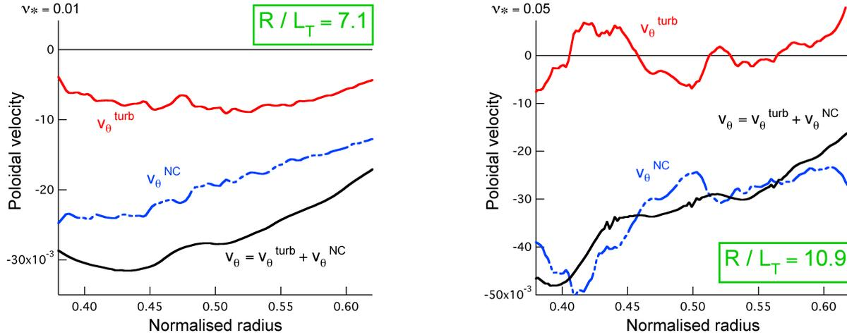
Figure 6: Poloidal velocity profiles in the turbulent regime for  $\nu_* = \{0.01, 0.05\}$  and  $R/L_T$ . The turbulent and neoclassical contributions are also plotted.
