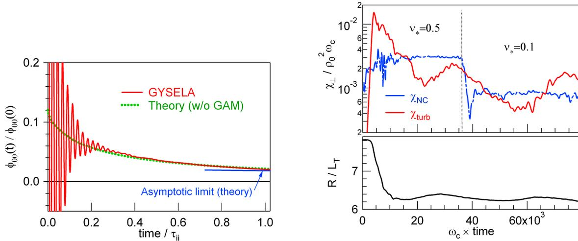
Figure 5: (left) Time relaxation of the poloidal  $E \times B$  flow initiated in GYSELA due to Landau damping and collisions. (right) Time traces of the turbulent and neoclassical heat flux and of  $R/L_T$  when  $\nu_*$  is decreased from 0.5 down to 0.1 at  $\omega_c t = 36.10^3$ .
